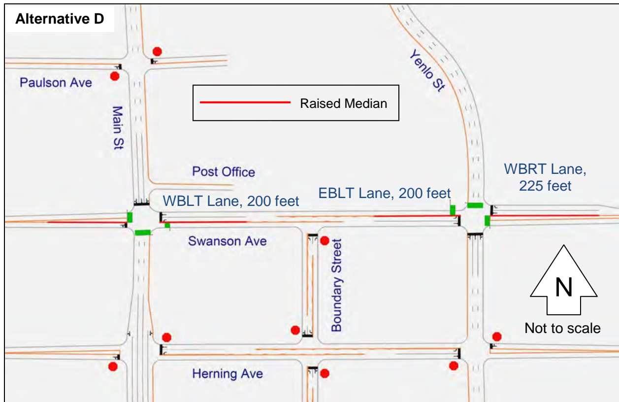
Figure 29: Auxiliary Lane Recommendations for Swanson Avenue Intersections, Alternative D
